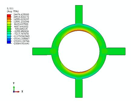
Figure 9: shows stress distributions adding the thermal part for number of elements 16997.
