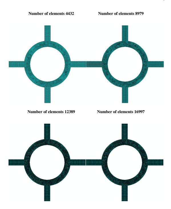
Figure 5: shows coarse, medium, and fine mesh for the same family of grid.
