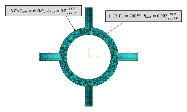
Figure 3: Quad-dominated mesh using first boundary conditions.
