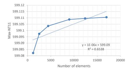
**Figure 6:** Grid Convergence for the pipe with fines.
