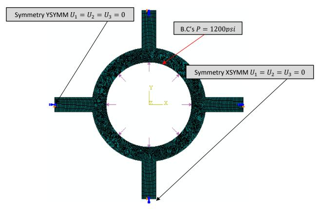
**Figure 4:** Quad-dominated mesh using second boundary conditions for number of elements 16997.
