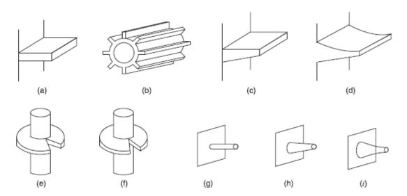
**Figure 1.** Schematic Diagrams of Different Types of Fins: (a) Longitudinal Fin of Rectangular Profile; (b) Cylindrical Tube with Fins of Rectangular Profile; (c) Longitudinal Fin of Trapezoidal Profile; (d) Longitudinal Fin of Parabolic Profile; (e) Cylindrical Tube with Radial Fin of Rectangular Profile; (f) Cylindrical Tube with Radial Fin of Truncated Conical Profile; (g) Cylindrical Pin Fin; (h) Truncated Conical Spine; (i) Parabolic Spine.
