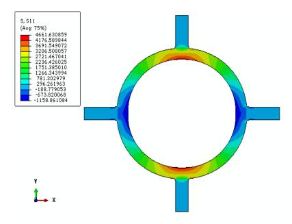
**Figure 8:** stress distribution for number of elements 16997.
