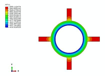
**Figure 7:** temperature distribution for number of elements 16997.
